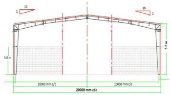
Fig .1 Single Frame of a Pre Engineered Building
